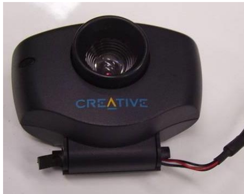
Figure 3: The Visual Vector Sensor webcam is a low-resolution off-the-shelf webcam that has been incorporated into the attitude determination system of the tabletop spacecraft simulator.
