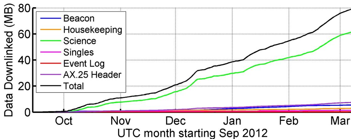
Figure 6: Cumulative data received from CSSWE. CSSWE uses five primary packet types: beacon, housekeeping, science (binned REPTile data + attitude data), singles (raw detector hits), and event log. Each packet uses an AX.25 header of identifying information.
