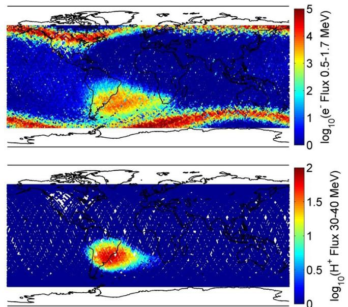
Figure 3: Measurements of 0.5 to 1.7 MeV electrons (top) and 30 to 40 MeV protons (bottom) from the REPTile instrument onboard CSSWE. The data were collected from October 5, 2012 to October 25, 2012.
