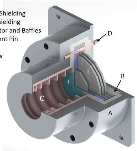
Figure 2: Solid model of the REPTile instrument with components labeled.
