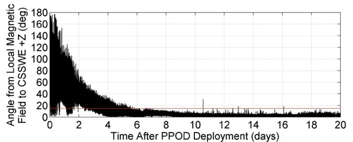
Figure 12: The angle between the local magnetic field and the CSSWE Z-axis is shown over the first 20 days on-orbit. The red line indicates an angle of  $15^\circ$ . CSSWE converged to within  $15^\circ$  of the magnetic field one week after orbit insertion.
